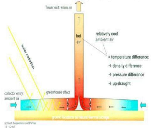
Fig 2: Operational Principle of Solar Updraft Tower
