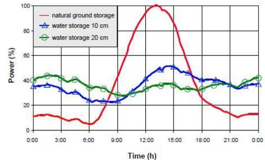
**Fig 3: Effect of using water filled tubes under collector roof**
